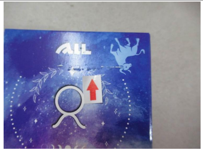
12. Defect-Glue mark on surface-minor
