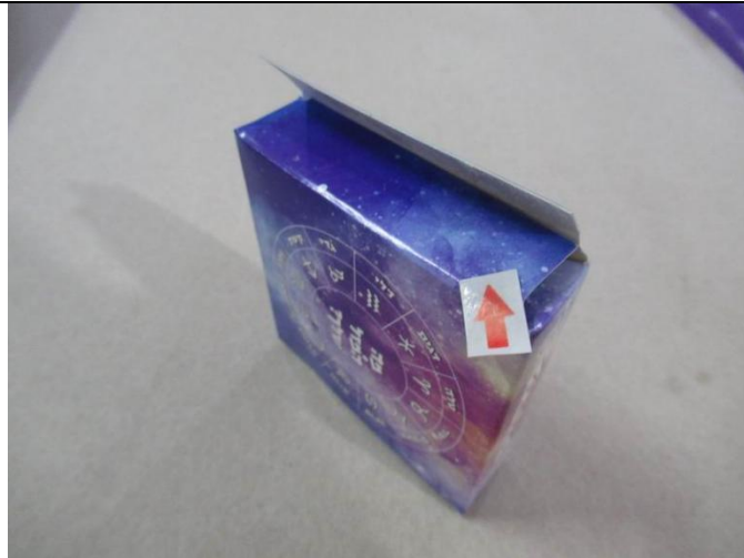
1. Defect-Poor glued of gift box-major
