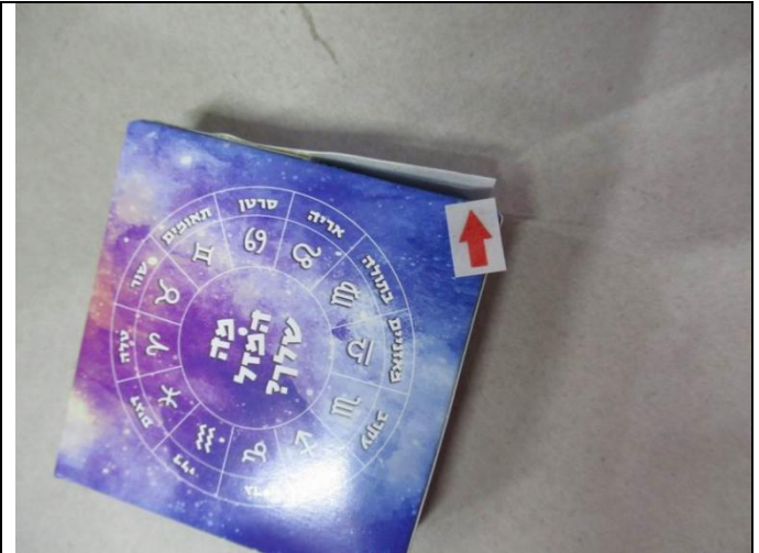
2. Defect-Poor glued of gift box-major
