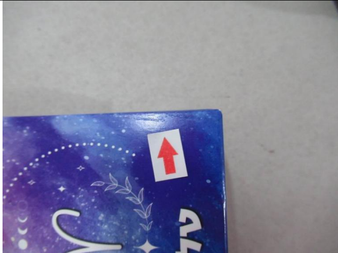
11. Defect-Glue mark on surface-minor
